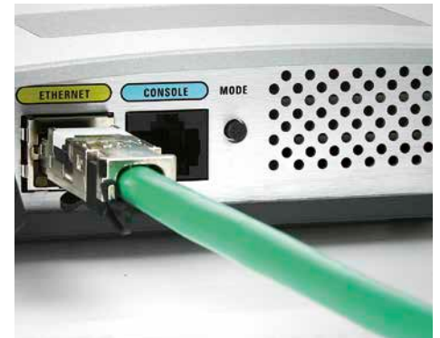
Fig. 3: Direct connection of a network device
