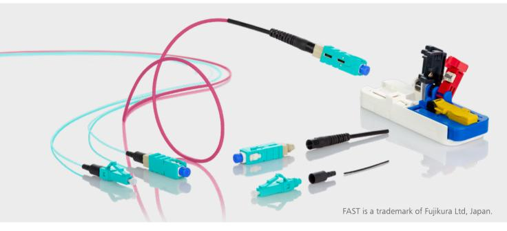
The OpDAT FAST<sup>TM</sup> connector is a field installable fibre optic connector for multi-mode technology that offers very good and constant optical transmission values. The FO connector can be assembled quickly and easily in the field - no gluing, no polishing and no special tools required. The factory-polished ceramic ferrule guarantees very good and stable connection
