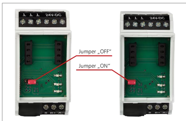
Figure 18 Password- jumper settings
