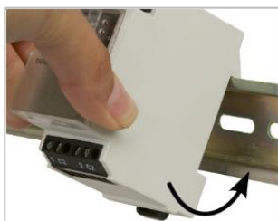
Figure 1 Mounting of MR-GW
